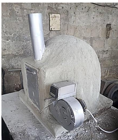
Fig. 11. Produced earthen oven.
